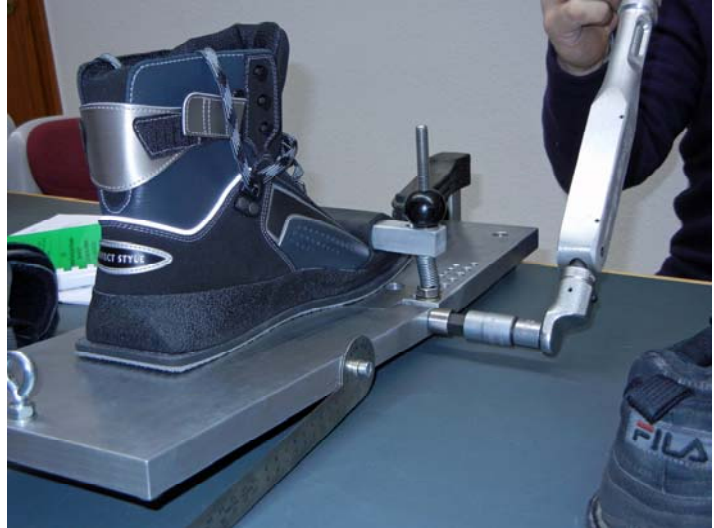
The new shooters' shoe testing device approved by the ISSF Technical Committee.
