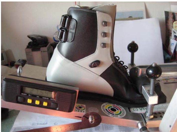
The new ISSF shoe testing device gives precise measurements of the flexibility of the shoe soles.
